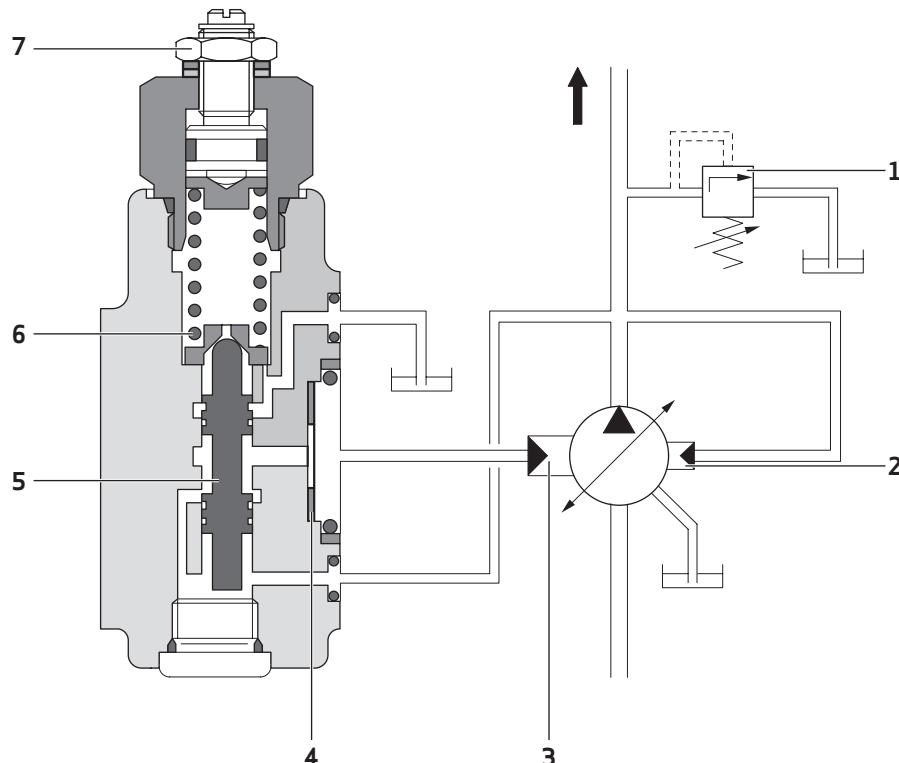
1 Safety valve  $p = p_{\text{maximum}} + 30 \text{ bar}$  (435 psi)
