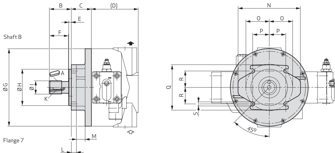
Involute spline to DIN 5480 (obligatory with multiple arrangement of RKP and SAE-B)
