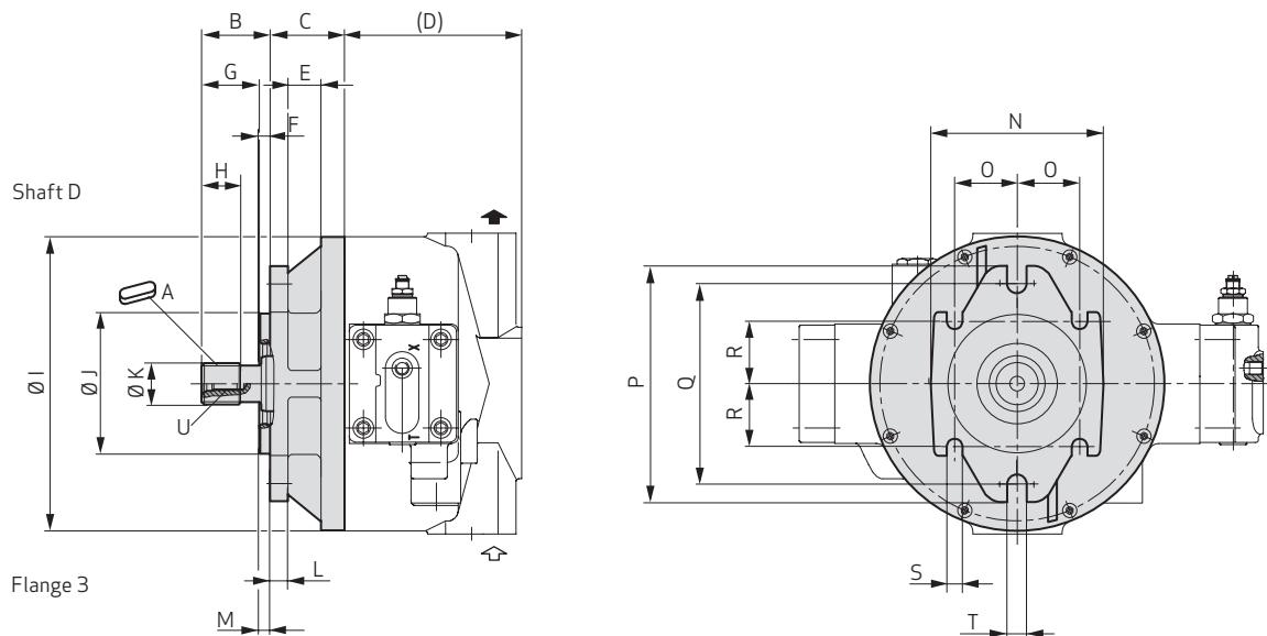
Involute spline to SAE 744 C, (obligatory with multiple arrangement of RKP and SAE-B)
