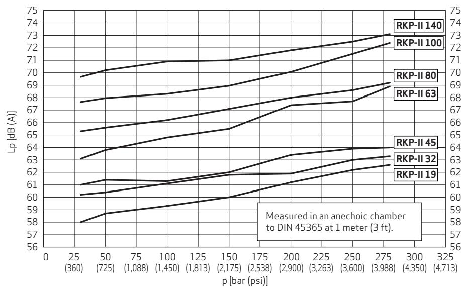
Noise emission values with combined pressure/flow compensator. These are average values over the operating range.
