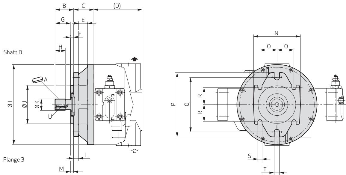
Key to SAE standard, SAE mounting flange to ISO 3019/1 (imperial dimensions)
