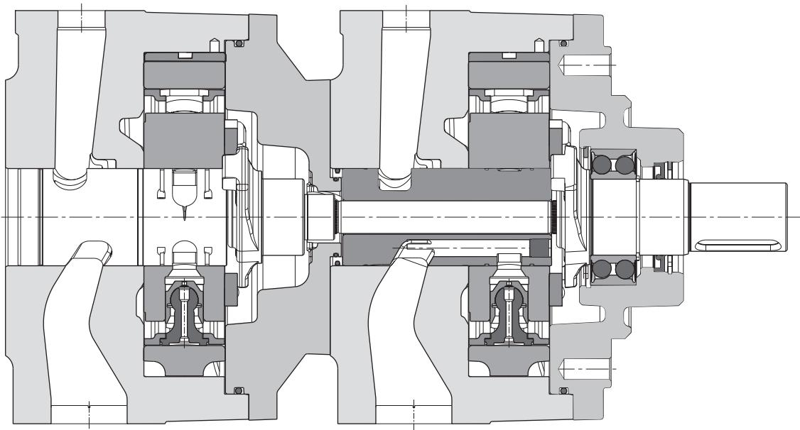
Radial piston pump with tandem mounted gear pump using SAE-A adapter. Technical data [see page 56](#).
