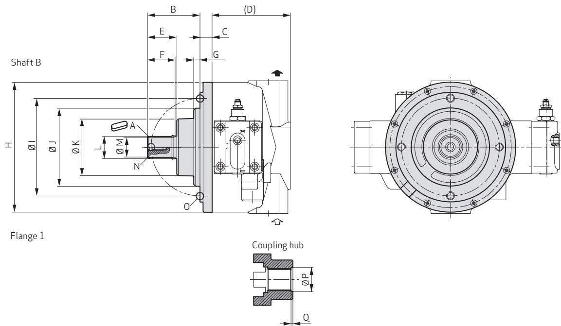
Involute spline to DIN 5482 (for B1), (obligatory with multiple arrangement of RKP and SAE-B), Metric round flange
