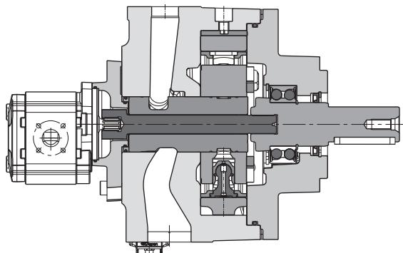
Radial piston pump with tandem mounted gear pump using SAE-B adapter. Technical data [see page 57](#).
